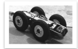
Sewer Inspection Equipment
