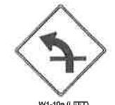
W1-10a (LEFT) HORIZONTAL ALIGNMENT SIGN DETAIL NOT TO SCALE
