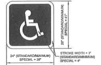
HANDICAP STRIPING DETAIL NOT TO SCALE (MARCH 2008)
