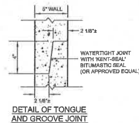
PRECAST REINFORCED CATCH BASIN NOT TO SCALE (MAY 2012)
