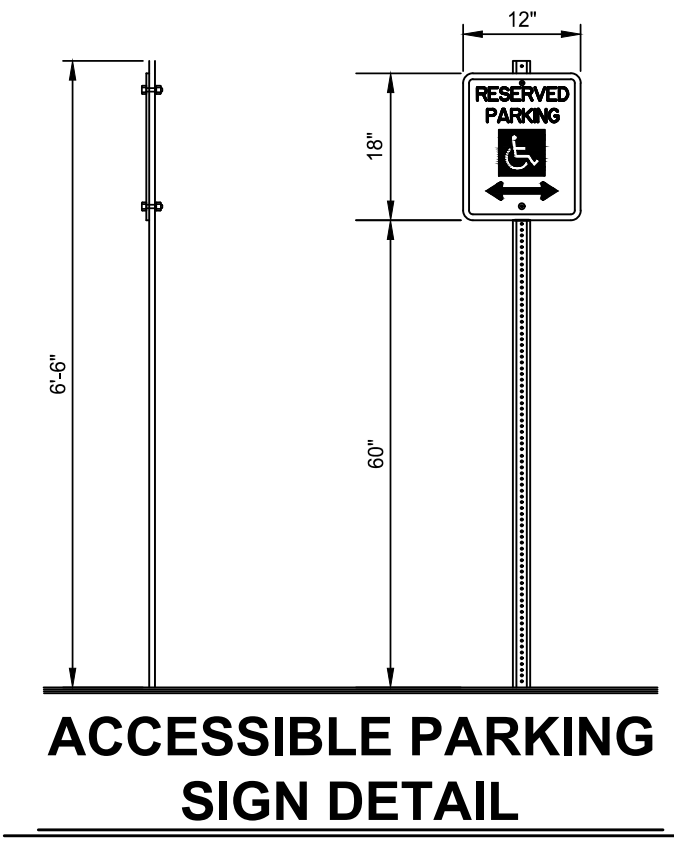
TRAFFIC SIGN SUPPORT DETAIL NOT TO SCALE
