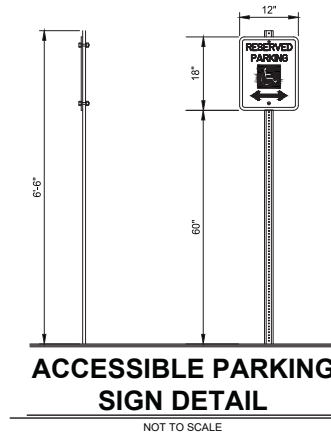
SECTION P2-10, P2-11 LENGTH: P2-10, 10'-0", P2-11, 11'-0" WEIGHT PER LINEAR FOOT: 3.00 LBS HOLES: 3/8" DIA. 1" C-C FULL LENGTH STEEL: SHALL CONFORM TO ASTM A-499 (GRADE 60) OR ASTM A-5761 (GRADE 1070-1080). FINISH: SHALL BE PAINTED WITH TWO COATS OF BAKED ON OR AIR DRIED, PAINT OF WEATHER RESISTANT QUALITY. ALL FABRICATION SHALL BE COMPLETE BEFORE PAINTING. PAINT SHALL BE SUBJECT TO THE APPROVAL OF THE ARCHITECT. SECTION P-11 THRU P-16 LENGTH: P-11, 11'-0", P-12, 12'-0", P-14, 14'-0", P-16, 16'-0" WEIGHT PER LINEAR FOOT: 3.00 LBS STEEL: SAME AS FOR P2-10, P2-11 FINISH: SAME AS FOR P2-10, P2-11 DIMENSIONS SHOWN ARE NOMINAL. ALTERNATE SECTIONS MUST BE APPROVED PRIOR TO USE. TRAFFIC SIGN SUPPORT DETAIL NOT TO SCALE
