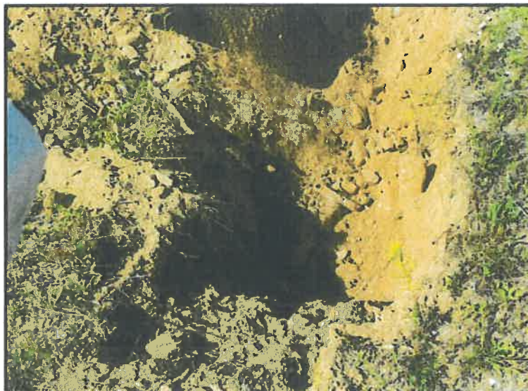
A view of the deeper sandy cobbly fill over natural sandy soil materials of the 550 disturbed soil map unit as described doing machine dug test pits.
