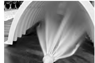
Examples of culvert cleaning nozzles appropriate for Isolator Row maintenance. (These are not StormTech products.)
