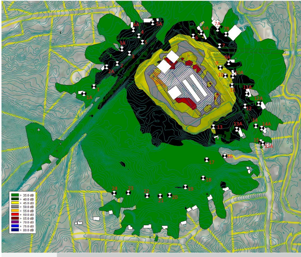
Figure 11. Noise Contour Map of the Forklift and Truck Noise.
