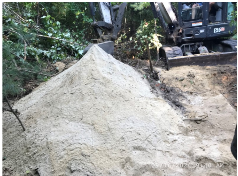
9-16-2024: Test Pit 2 spoil pile, note loamy sand with few coarse fragments found at bottom of pit in C horizon (top of pile).
