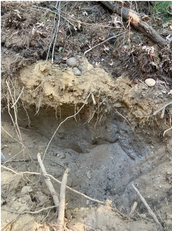
9-16-2024: Test Pit 1 (stratified coarse sand with gravel)
