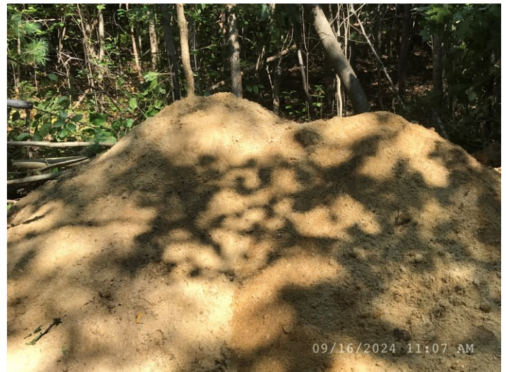
9-16-2024: Test Pit 4 spoil pile, note nice medium sand
