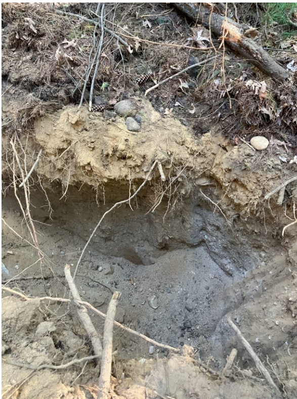
9-16-2024: Test Pit 1 (stratified coarse sand with gravel)
